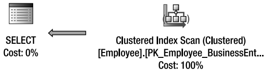
Figure 8-3. Base execution plan with scan on the clustered index
