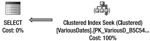
Figure 11-2. Querying date/time columns CAST to date type allows the query engine to take advantage of an index seek.
