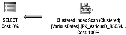
Figure 11-1. Converting the date/time column to a string does not result in a good execution plan.
